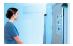
Metrasens's Ferroguard Assure safety system detects risk items 'well before they reach the MRI doorway', while Ferroguard Screener 'detects the smallest ferrous items' (e.g. hair-pins) on patients, 'reducing image artefacts, time-wasting rescans, and resulting reductions in efficiency'.
