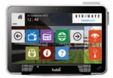
interaction. The device replaces the standard mouse, allowing users to navigate and control a computer using only their eyes."
